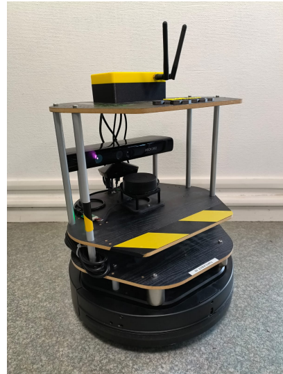
Figure 1. The robot we used for experiments. It is a modified Turtlebot 2 equipped with a Jetson Nano computer running ROS2, a Kinect depth camera and a RPLIDAR A1 2D LiDAR.
